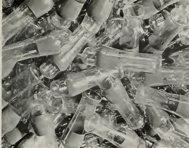
PART OF THE MILLIONS OF GLASS ENVELOPES AWAITING THE NEXT STEP IN TUBE MANUFACTURE AT THE RCA PLANT, HARRISON, N. J.
